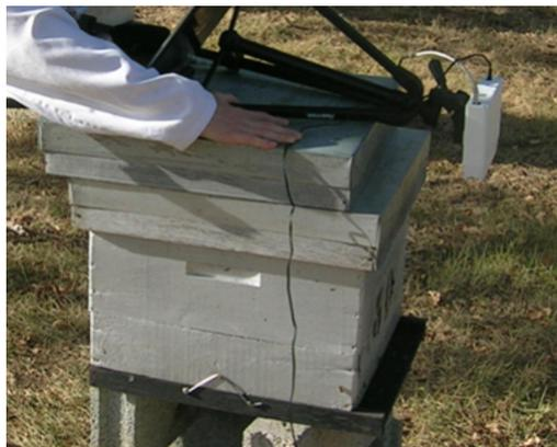
**Figure 2: Stereo vision camera.** A stereo vision camera capturing the entry of a beehive including the entire flight board.
