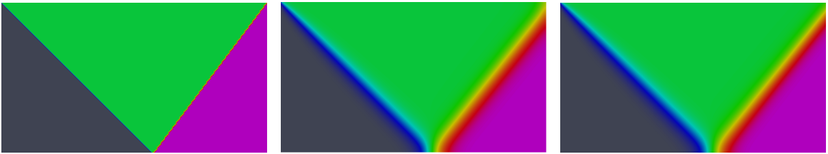
Figure 2. Shock reflection, mesh 140 \times 80 . Exact solution (left), Lattice Boltzmann scheme D2Q5Q4Q4 (middle) and Godunov scheme (right).
