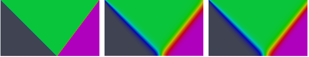
Figure 2. Shock reflexion, mesh 140 \times 80 . Exact solution (left), Lattice Boltzmann scheme D2Q5Q4Q4 (middle) and Godunov scheme (right).
