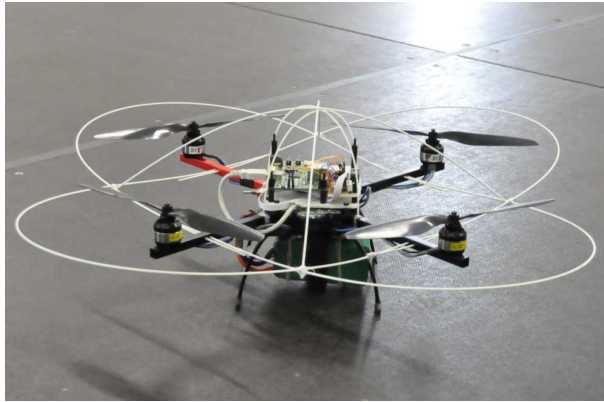
Fig. 10 MAV experimental platform: The quad-rotor equipped with imaging, inertial and altitude sensing systems.
