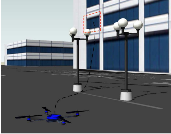
Fig. 1 Scheme of the MAV application. The vehicle should compute a trajectory with obstacle avoidance capabilities using a vision system and GPS information.
