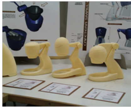
FIGURE 1.5: Example of physical prototypes from hand-made sketches (courtesy of Eiger).
