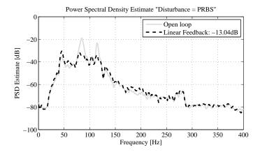
Figure 6: Power spectral density of the open loop and when using the fixed feedback controller.
