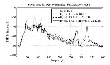
Figure 10: Power spectral density of the adaptive filters.
