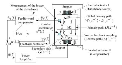
Figure 2: An AVC system using an adaptive feedforward and a fixed feedback compensation scheme.
