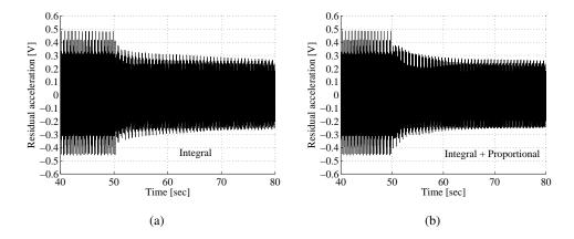
Figure 13: Real time results obtained with Algorithm  $I_L$  using (a) "Integral" scalar adaptation gain and (b) "Integral + Proportional" scalar adaptation gain.
