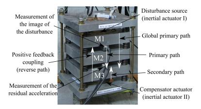
Figure 1: The AVC system used for experimentations - photo.
