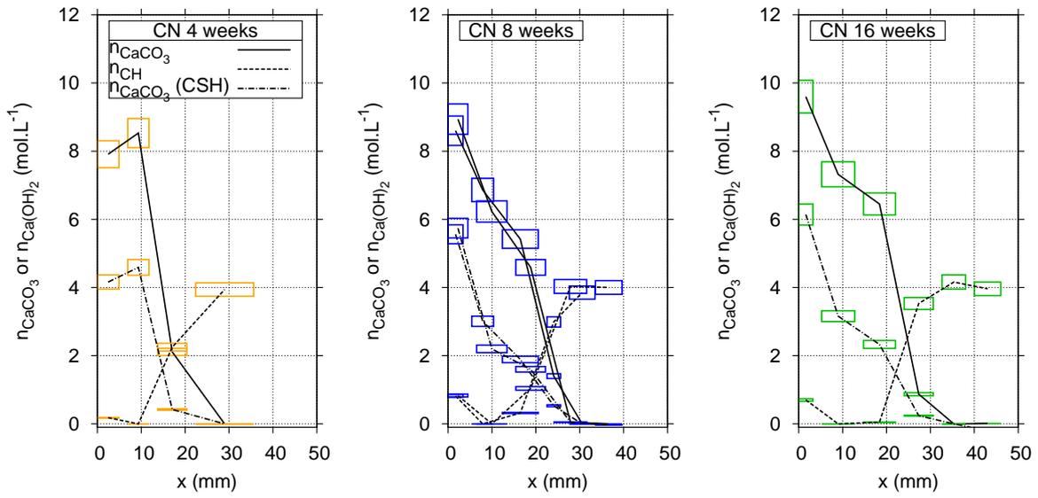
Figure 13: Carbonation profiles assessed by TGA-MS. Illustration of contents of CH and  $\bar{C}\bar{C}$  (for  $\bar{C}\bar{C}$ , total content and content only related to C-S-H carbonation are illustrated) after 4, 8 et 16 weeks of exposure to  $\text{CO}_2$ . Case of CN paste. For the case of 8 weeks of exposure, the profiles for two different specimens are shown.
