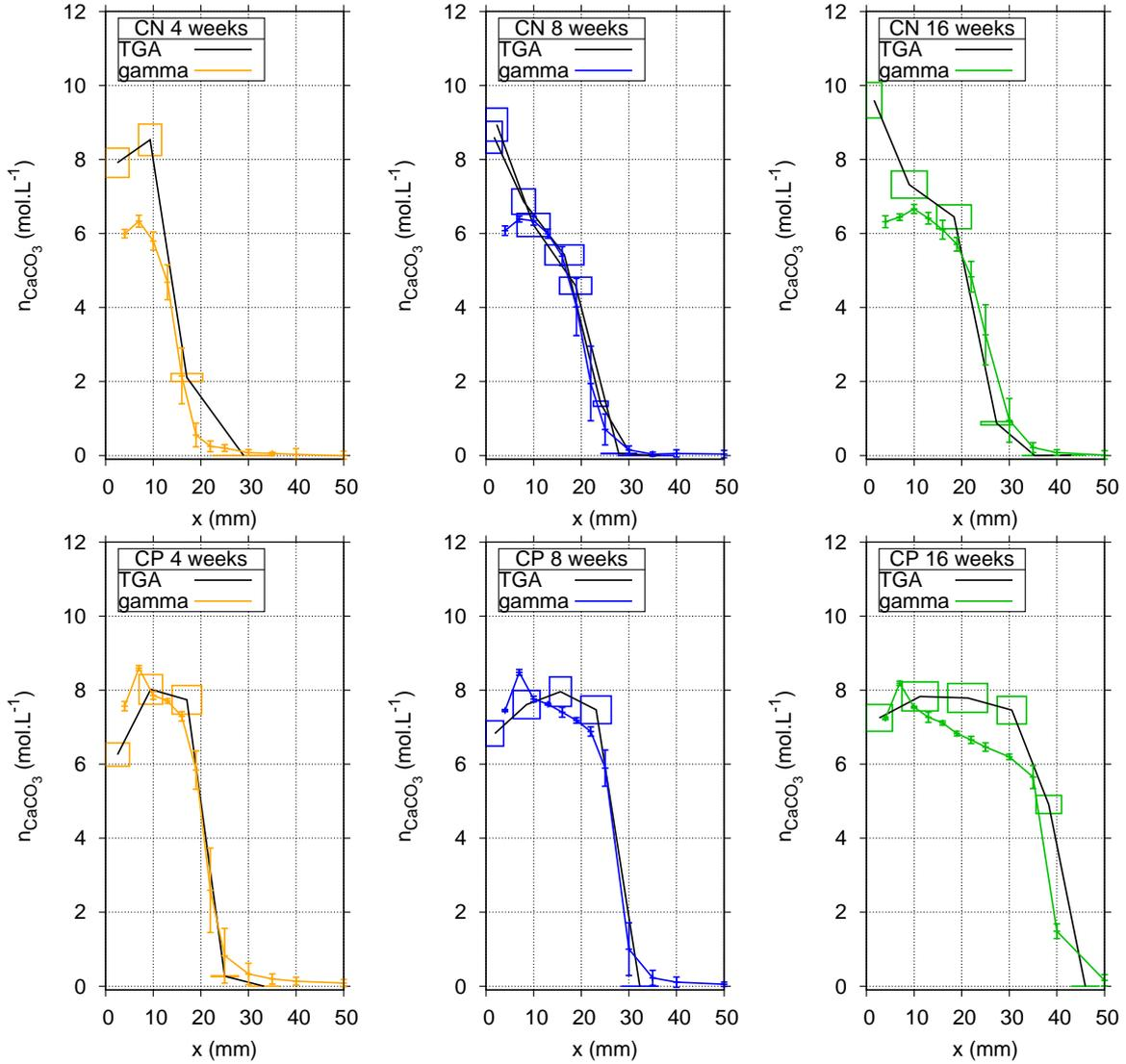
Figure 15: Assessment of CO<sub>2</sub> fixed to the cement matrix as  $\overline{C\overline{C}}$  ( $n_{\overline{C\overline{C}}}$ ) for CN and CP after 4 (orange), 8 (blue) and 16 (green) weeks of accelerated carbonation. TGA-MS data are represented by coloured boxes while GRAM data are represented as coloured lines.
