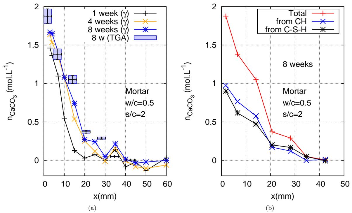
Figure 17: (a) Content of the  $\text{CO}_2$  fixed to the cement matrix as  $\text{C-C}$  are represented for the studied mortar (CEM I cement,  $w/c=0.5$  and  $s/c=2$ ). TGA results are represented by coloured boxes while GRAM are represented as coloured lines. (b) Quantification of total  $\text{C-C}$  (red) and balance between  $n_{\text{C-C}}^{\text{CH}}$  (blue) or  $n_{\text{C-C}}^{\text{CSH}}$  (black) after 8 weeks of carbonation for the mortar
