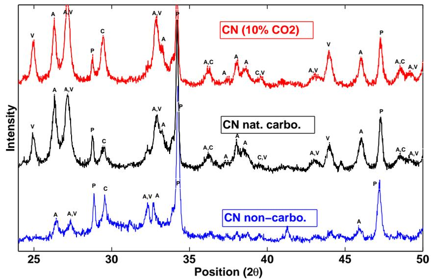
Figure 12: Comparison of XRD patterns for non-carbonated and carbonated (natural conditions and  $\text{CO}_2=10\%$ ) CN samples. A for aragonite, V for vaterite, C for calcite and P for portlandite.
