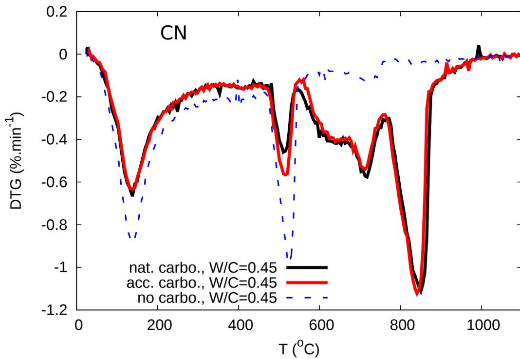
Figure 11: Comparison of DTG diagrams between non-carbonated and carbonated CN (10% CO<sub>2</sub> or natural carbonation).
