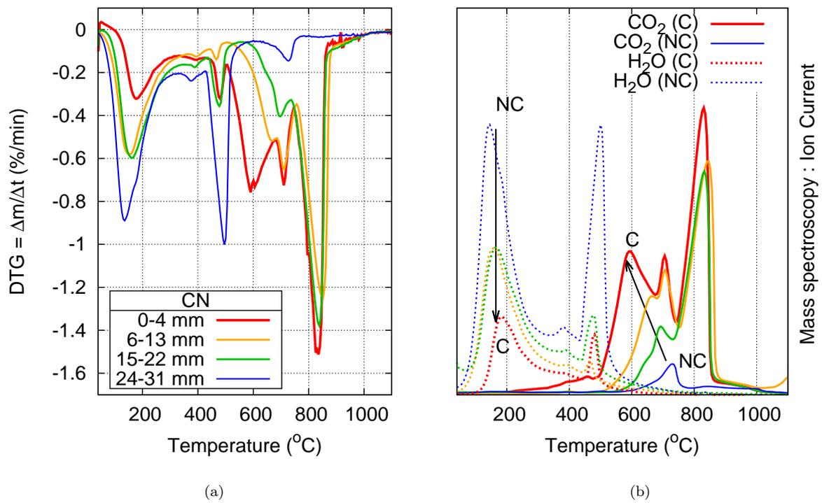
Figure 9: Diagrams of thermal analysis of samples sawn from the surface exposed to CO<sub>2</sub> to the core of a CN specimen exposed to 10% CO<sub>2</sub> during 8 weeks. (a) DTG diagrams and (b) mass spectroscopy diagrams.
