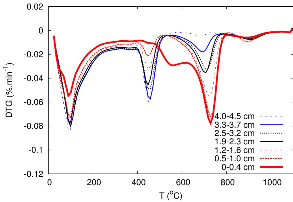
Figure 10: DTG diagrams of the slices sawn from the mortar specimen exposed to 10% CO<sub>2</sub> during 6 weeks.
