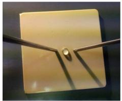
Figure 2b: Coplanar inclined cylindrical electrode configuration.
