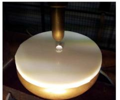
Figure 2a: Rod to plane electrode configuration with a circular silicon sample.
