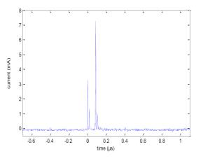
Figure 4a: Typical current detected for  $30\mu$ l volume droplet at 28 kV for 11mm inter-electrode distance in rod to plane system.
