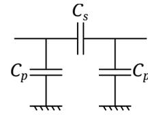
Figure 3. Equivalent  $\pi$  network of the proposed topology.
