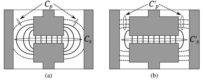
Figure 4. Solid lines represent the series capacitance  $C_s$  and dash lines the capacitance with the ground  $C_p$ . For small widths, the most part of the fringing field is between the plates (a). When the width of the plates increase, the ground catches a part of the fringing field:  $C_s$  reduces and  $C_p$  grows (b).
