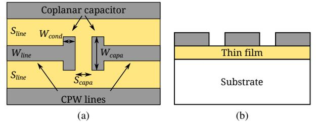
Figure 1. Proposed topology to extract complex permittivity. In practice,  $W_{line} = 30 \mu\text{m}$ ,  $S_{line} = 150 \mu\text{m}$ ,  $W_{cond} = 30 \mu\text{m}$ ,  $W_{capa} = 60$  to  $150 \mu\text{m}$  and  $S_{capa} = 4$  to  $12 \mu\text{m}$ . The thin film thickness is  $1 \mu\text{m}$ .
