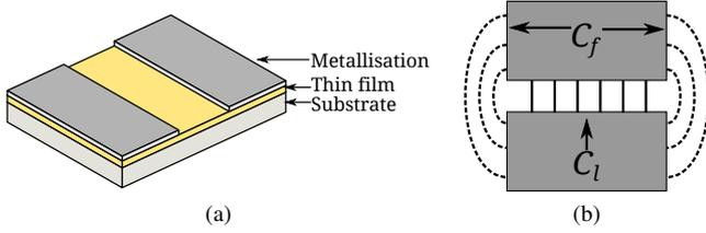
Figure 2. Topology describes by Vendik's model. Solid lines represent the linear capacitance  $C_l$  and dash lines the fringing field capacitance  $C_f$  at the plates extremities. The model only considers the contribution of the linear capacitance  $C_l$ .
