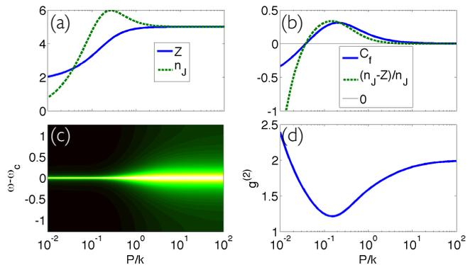
FIG. 2: Subradiance and superradiance for 5 emitters in the bad cavity regime,  $g = 0.1k$ . (a) Total atomic inversion,  $Z$ , and average value of the total atomic dipole,  $\langle J^\dagger J \rangle$ ; (b) Cooperative fraction compared to  $(n_J - Z)/n_J$ ; (c) Cavity spectrum; (d) Second-order coherence function  $g^{(2)}(0)$ . All the data are plotted as a function of the pump rate.
