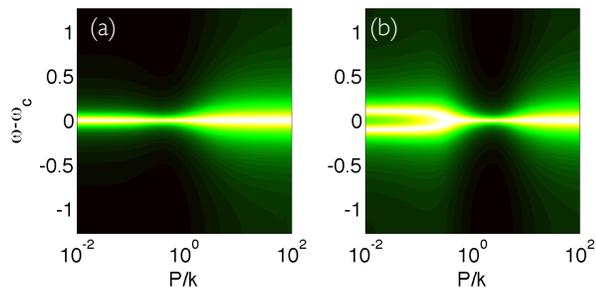
FIG. 4: The spectral signature of superradiance-lasing crossover for 4 emitters coupled to the same cavity mode: spectrum of the emitted radiation vs. pumping rate for (a)  $g = 0.2k$ , and (b)  $g = 0.5k$ , respectively.
