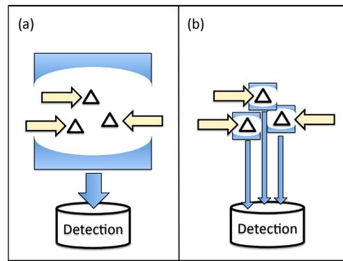
FIG. 1: The system under investigation, and the operational definition of cooperativity.  $N$  emitters being incoherently pumped, two situations are compared. (a) A detector captures the output of a cavity containing the ensemble of emitters. (b) Each emitter is coupled to an individual cavity, and each output signal is assumed to be detected and summed.
