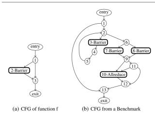
Figure 1: Examples of Control Flow Graphs
