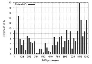
Figure 5: Execution-Time Overhead for EulerMHD (Weak Scaling)
