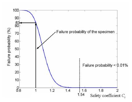
Fig. 7 Failure probability according to the safety coefficient  $C_{s.}$
