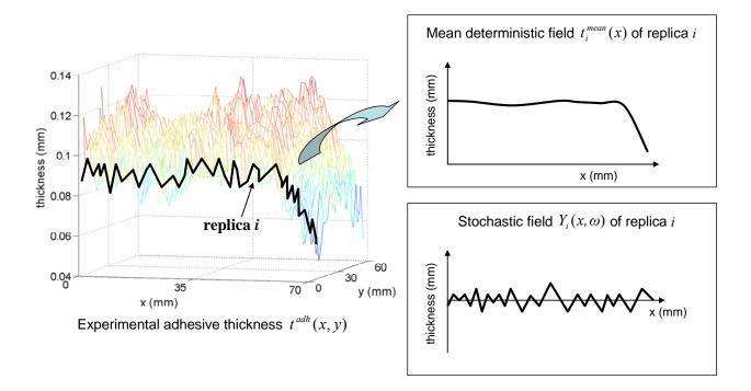
Fig. 2 Scheme of the decomposition of the experimental thickness  $t^{adh}(x,y)$ . The experimental thickness  $t^{adh}(x,y)$  presents two types of variations: the first is global and is represented by the mean deterministic field  $t_i^{mean}(x)$  for each measure in the x-direction; the second is modelled by a stochastic field  $Y_i(x,\omega)$  for each measure in the x-direction.
