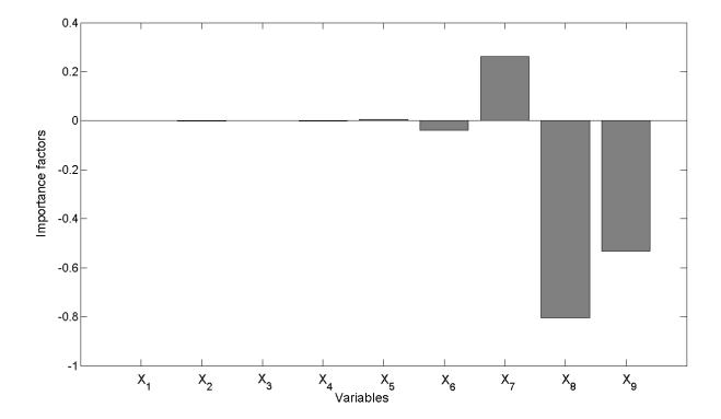
Fig. 6 Importance factors of the  $X_i$ - variables. The variables located near the free edge ( $X_7$ ,  $X_8$ ,  $X_9$ ) have significant importance factors. Therefore, their influences on the failure probability of the bonded joint are higher than the influences of the other variables.
