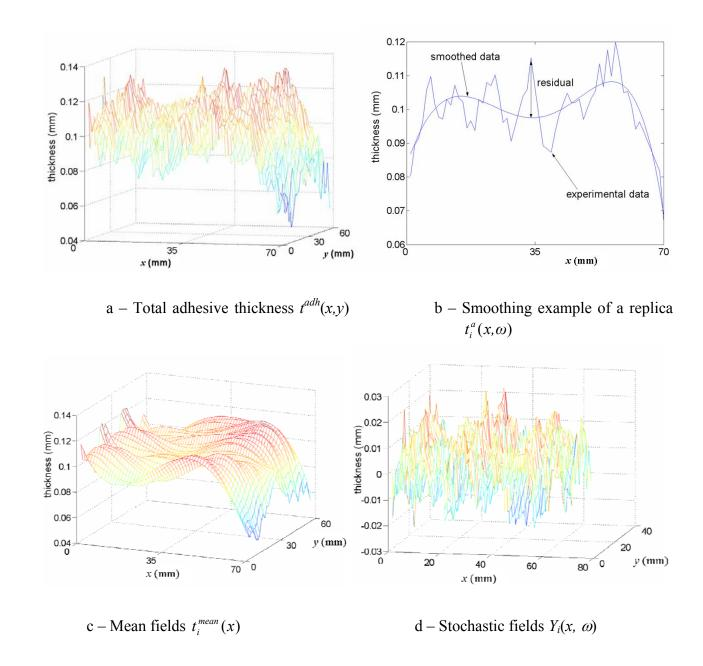
Fig. 3 Results of the adhesive thickness field decomposition  $t^{adh}(x,y)$ . Each measure  $t_i^a(x,\omega)$  in the x-direction is smoothed in order to obtain the mean fields  $t_i^{mean}(x)$ . Then, the stochastic fields  $Y_i(x,\omega)$  are obtained by subtracting the mean fields  $t_i^{mean}(x)$  from the adhesive field  $t^{adh}(x,y)$ .
