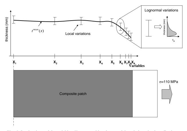
Fig. 5 Stochastic model: variables  $X_i$  are considered to model variations in the adhesive thickness. These variables follow a lognormal distribution and their abscissae are distributed according to a geometric distribution.
