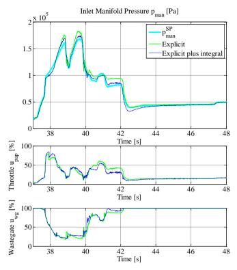
Figure 5. Inlet manifold pressure tracking performances for two explicit NMPC schemes : with and without anti-windup integral action on the throttle. Comparative actuators position graphs are depicted.
