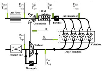
Figure 1. Air path sketch of a turbocharged SI engine (p stands for pressure, T for temperature,  $N_e$  and  $\omega_t$  are respectively the engine and turbocharger rotational speed).
