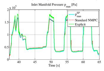
Figure 4. Inlet manifold pressure tracking performances for different NMPC schemes are depicted on the first graph. The standard NMPC uses iterative online optimization and the explicit NMPC is computed using the algorithm presented in the paper.
