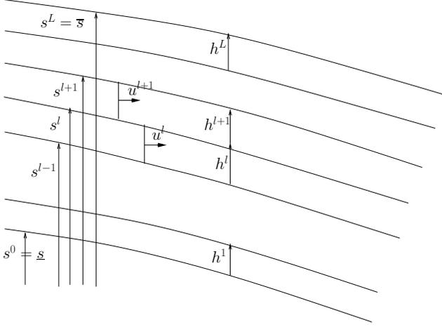
Figure 3: Multilayer splitting of the ice thickness.
