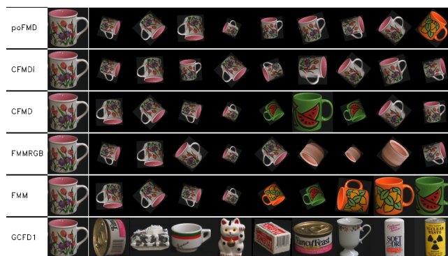
Figure 3: Modified COIL 100: nine best retrievals (ordered from left to right) for the query of the "colorful mug" (left column) with poFMD , CFMD , GCFD1 (parametrized by the bivector B_{red} ), CFMDi , FMM rgb and FMM .
