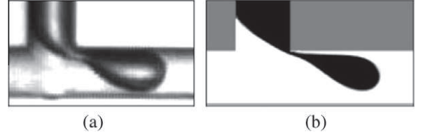
Fig. 11. Comparison of the bubble thread just before being squeezed in (a) experiments and (b) numerical simulations. U_{SL} = 0.318 m/s and U_{SG} = 0.081 m/s.
