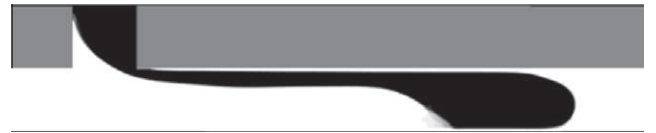
Fig. 8. Gas thread generation without squeezing. U_{SL} = 0.318 m/s and U_{SG} = 0.182 m/s.
