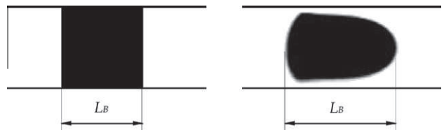
Fig. 21. (Left) bubble length given by Eq. (22), and (right) actual bubble length.
