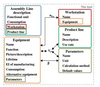
FIG. 3 – Organization of data and links between characteristics
