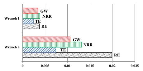
FIG. 5 – Comparison of normalized EI for two wrenches for the same functional unit (GW: global warming, NRR: non-renewable resources, TE: terrestrial ecotoxicity and RE: respiratory effects).
