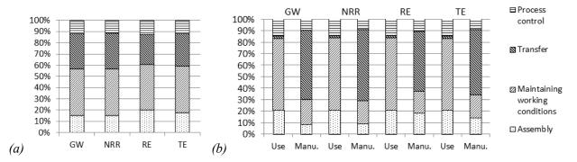
FIG. 6 – Proportion of each assembly line function in the overall assembly line EI (a); in the EI of the use. phase and manufacturing phase (b). (GW: global warming, NRR: non-renewable resources, TE: terrestrial ecotoxicity and RE: respiratory effects).
