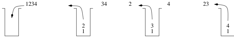
Figure 1: Four steps in the sequence of operations that outputs 2341 from 1234 using a stack. Each arrow shows an operation that is about to be performed.
