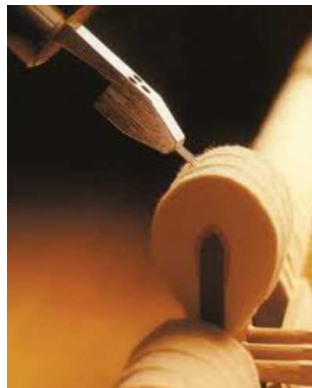
(b) Hammer voicing with a needle voicing tool. From piesikpiano.com.
