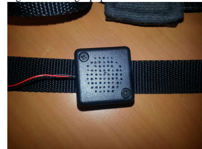
Fig. 5. Speaker attached to the harness
