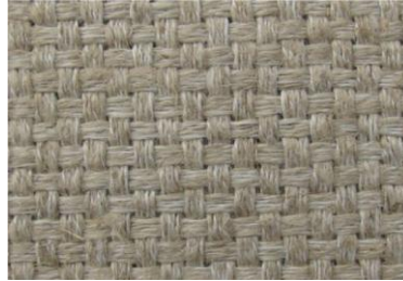
Figure 1 The 4x4 hopsack fabric
