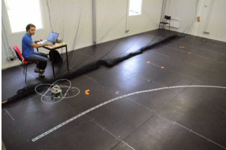
Fig. 19. Road-following mission: The rotorcraft flying in the experimental area during real-time tests.
