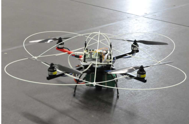
Fig. 5. UAV experimental platform: The quad-rotor equipped with imaging, inertial and altitude sensing systems.
