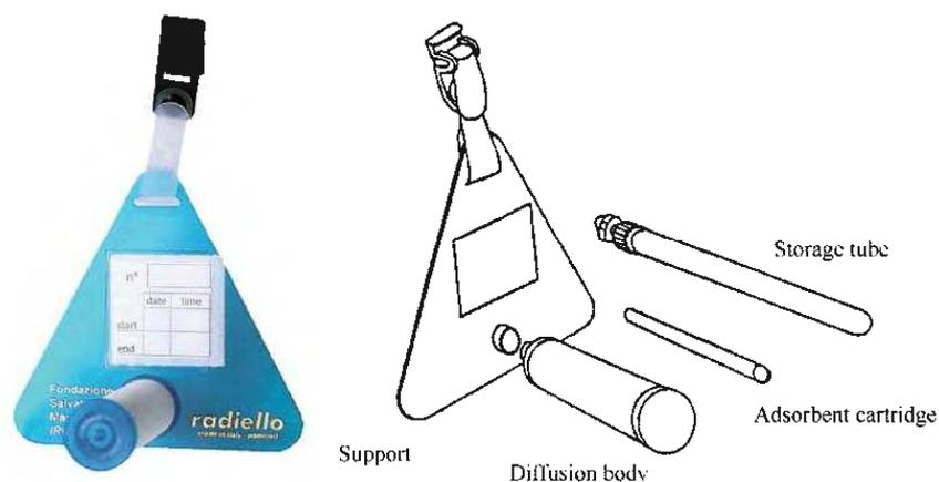
Fig. 1. Radiello diffusive sampler.
