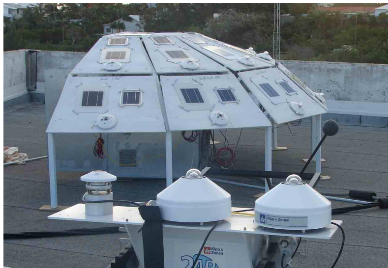
Fig. 1. Semi-hemispherical structure and sun tracker
