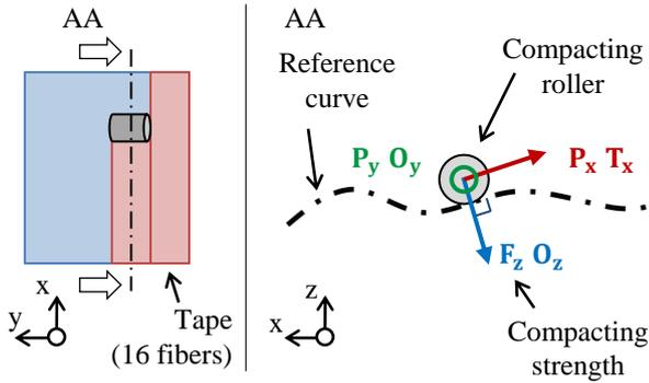
Fig.4. Dual command: force  $\mathbf{F}_{i\text{-axis}}$  vs position  $\mathbf{P}_{i\text{-axis}}$ , torque  $\mathbf{T}_{i\text{-axis}}$  vs orientation  $\mathbf{O}_{i\text{-axis}}$
