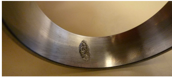
Figure 6: Defect on bearing outer-ring
