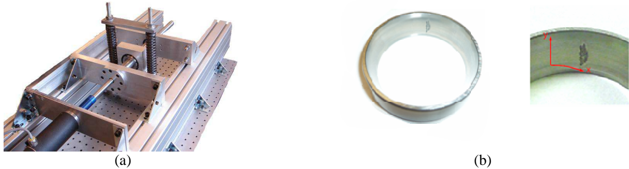
Figure4: (a) Specific test bench (b) Example of fault on bearing outer ring
