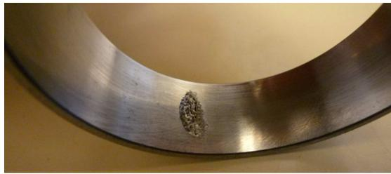
**Figure 6: Defect on bearing outer-ring**
