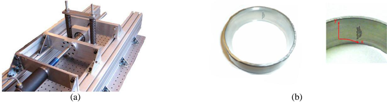
Figure4: (a) Specific test bench (b) Example of fault on bearing outer ring
