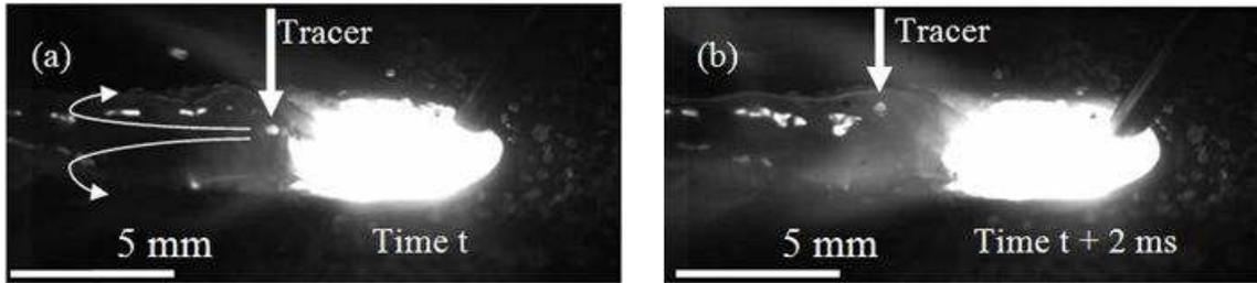
**Figure 11.** (a and b): Two images extracted from a video sequence showing the displacement of a tracer (indicated by an arrow) between a time interval of 2ms (MAG process: Welding speed  $U_0$ : 2 m/min; Wire speed  $V_w$ : 9 m/min). General trend of the melt flow surface is also indicated by curved arrows on figure 11-a.
