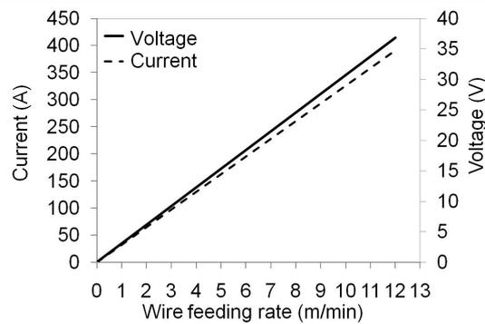
**Figure 3.** Voltage and current synergy obtained with the parameters of our study (S355 steel, 1.2 mm diameter wire, shielding gas: 92% Ar - 8% CO<sub>2</sub>).
