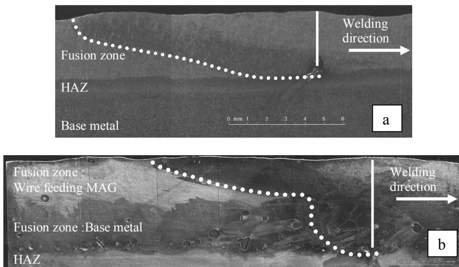
**Figure 14.** Longitudinal macrographs obtained with copper/aluminium alloy contrast material. The dotted line shows the melt pool boundary. Vertical white bar shows the initial position of the contrast wire. a- MAG alone ( $U_0=0,8$  m/min,  $V_w=5$  m/min). b- Hybrid laser/MAG ( $P_{laser}=4$  kW,  $U_0=1$  m/min,  $V_w=5$  m/min, wire/laser beam distance: 2 mm).
