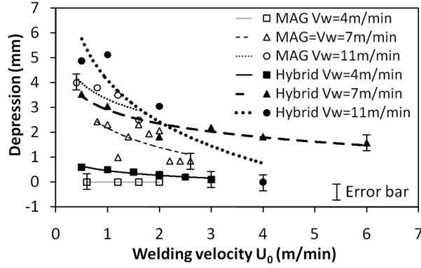
**Figure 9.** Maximum surface depression below the solid surface for MAG and Hybrid processes, as a function of welding speed for different wire feeding rates  $V_w$  (Hybrid parameters:  $P_{\text{laser}}$  : 4 kW, wire diameter : 1.2 mm, distance wire/beam: 2 mm).
