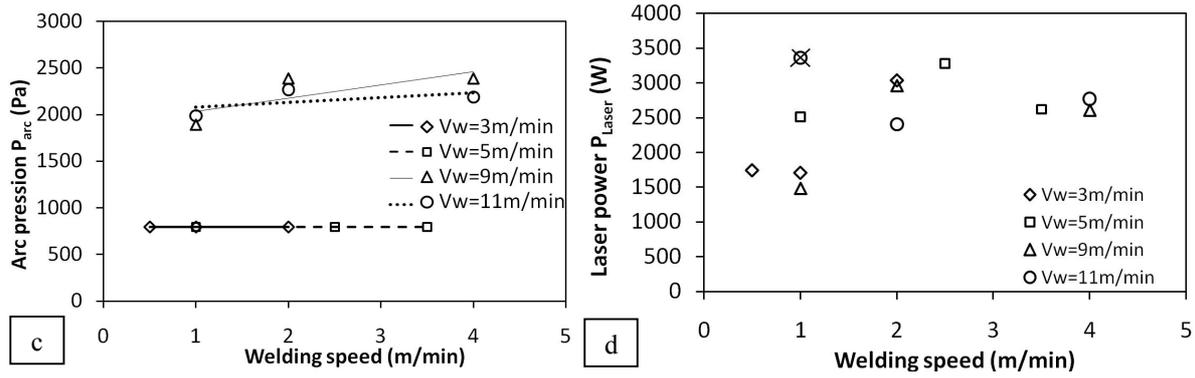
**Figure 17.** Parameters used in the simulation to reproduce the weld pool characteristics determined from macrographs and melt pool length measured using videos: arc efficiency (a), arc power radius (b), arc pressure (c) and laser power (d), obtained with hybrid Laser-MAG for different wire speeds.
