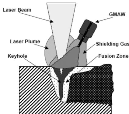
**Figure 1.** Scheme of hybrid laser – MIG/MAG process.
