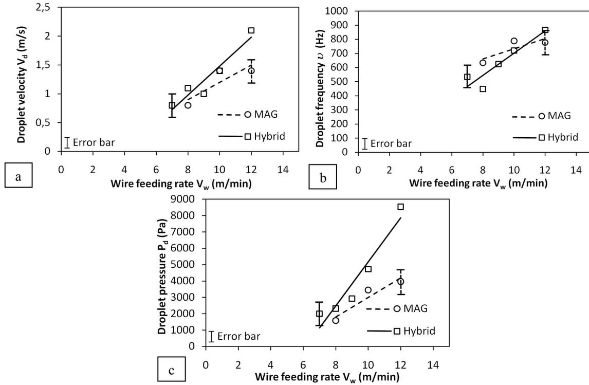
**Figure 10.** For Hybrid laser-MAG process, (a) droplet velocity, frequency (b) and (c) induced pressure (given by equation 1), as a function of the wire feeding rates.
