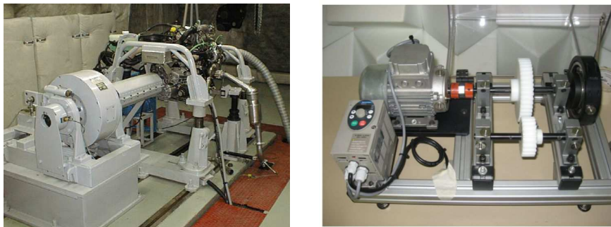
Fig. 2. Test rigs used for signals and results shown in this work. Left : Diesel engine, right : gears.
