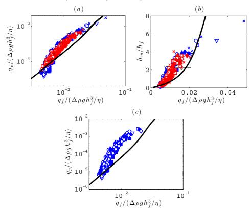
FIGURE 11. (a) and (b) Same as figure 6 and (c) particle flux  $q_p/(\Delta \rho g h_f^3/\eta)$  with comparison to the two-phase model using the suspension rheology of Boyer *et al.* (2011) (2D: solid line).
