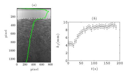
FIGURE 2. (a) Averaged image after 35.5 s for run 2 with the corresponding averaged grey-level profile (-, green on line) and detected fluid-bed interface (--, white on line). (b) Temporal evolution of the fluid height  $h_f$  for the same run.
