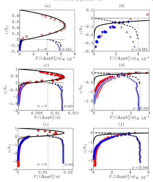
FIGURE 12. Same as figure 7 but with comparison to the two-phase model using the suspension rheology of Boyer *et al.* (2011) (2D: solid line). The variation of  $\phi$  along z is also represented (blue +: experiments and black dashed line: 2D predictions).
