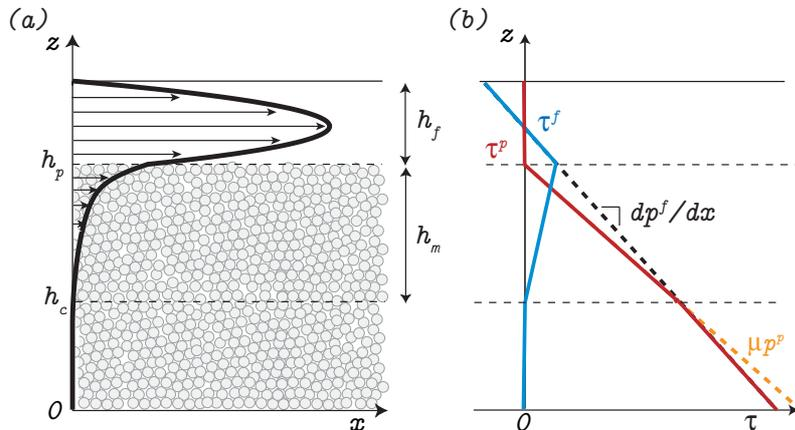
FIGURE 4. Sketches (a) of the particle bed submitted to a Poiseuille flow and (b) of the exchange between the fluid  $\tau^f$  (blue online) and particle  $\tau^p$  (red online) stresses inside the granular bed.
