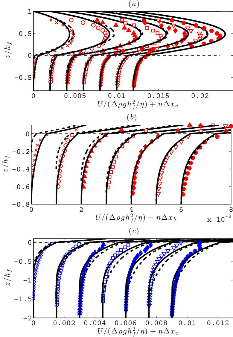
FIGURE 10. Comparison of the dimensionless velocity profiles between experiments corresponding to the different locations of (a, b) run 15 for  $h_f = 16.7$  mm and (c) run 5 for  $h_f = 8.1$  mm (symbols in table 2) and theoretical two-phase model using the granular rheology (2D: black dashed line and 3D: black solid line). The plots are shifted for clarity ( $\Delta x_a = 0.002$ ,  $\Delta x_b = 0.001$ ,  $\Delta x_c = 0.0015$ ). Graphs (b) is a blow-up of graph (a).
