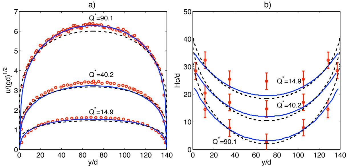
Figure 10: Granular flow on a heap. a) Surface velocity profiles; b) Depths of the flowing layer across the channel width. Present numerical results (mesh of  $1 \times 70 \times 100$  H27 FE on the half domain,  $\lambda_p = 10^{-7}$ ,  $\lambda_r = 10^{-5}$ , dashed line - -), numerical solutions from Jop *et al.* [20] (grid size of  $71 \times 80$  on the full domain, solid line —) and experimental results from Jop *et al.* [19] (circles  $\circ$ ).
