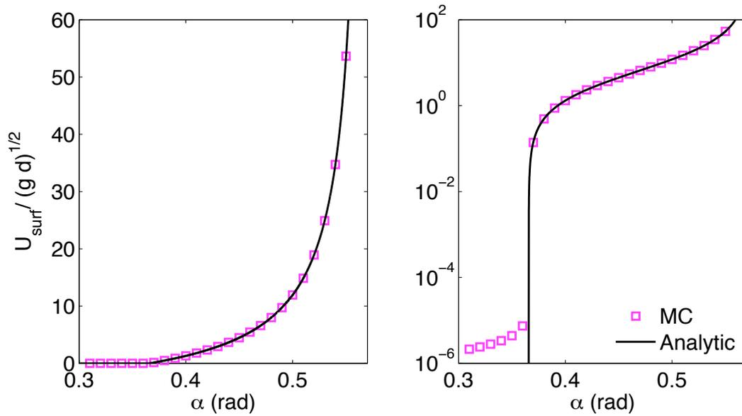
Figure 8: Granular flow over an inclined rough plane for  $H = 14$ . Comparison between numerical ( $h = H/80$ ,  $\square$ ) and analytical (solid line) free surface velocity  $u(z = H)$  as a function of the tilt angle  $\alpha$ .
