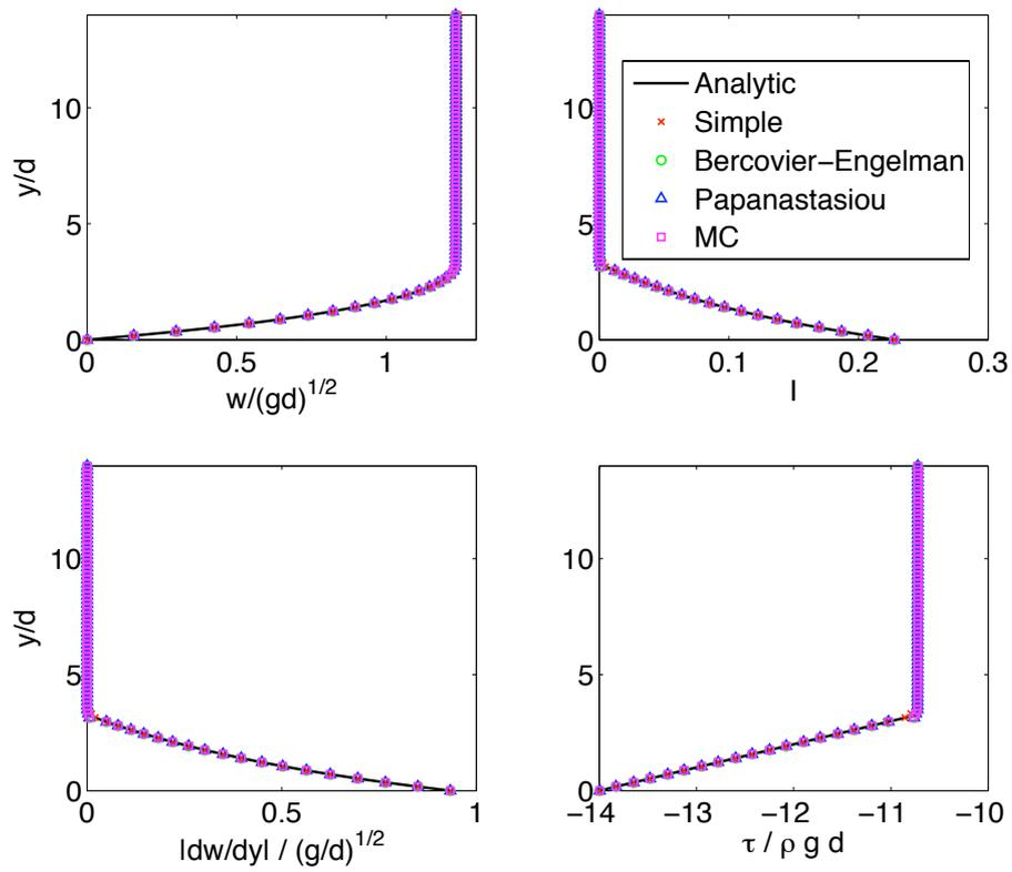
Figure 2: Vertical-chute flow test case with  $p = 28$  and  $b = 28$ . Comparison of computed ( $h = b/80$ ) and analytical solution profiles: vertical velocity component  $w$  (upper left), transverse velocity gradient  $dw/dy$  (lower left), inertial parameter  $I$  (upper right) and shear stress  $\tau$  (lower right).
