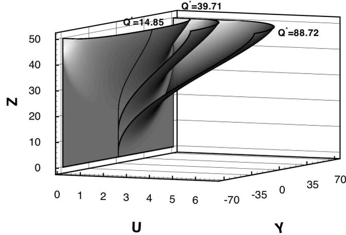
Figure 11: Velocity profiles obtained with the present model (Grid size:  $1 \times 70 \times 100$ , half domain, penalisation parameter:  $\lambda_p = 10^{-7}$  and regularisation parameter:  $\lambda_r = 10^{-5}$ ) for three different dimensionless flow rate ( $Q^* \in \{14.85 ; 39.71 ; 88.72\}$ ).
