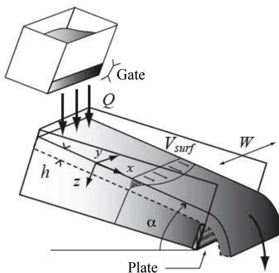
Figure 9: Sketch of the heap-flow experimental configuration [19]
