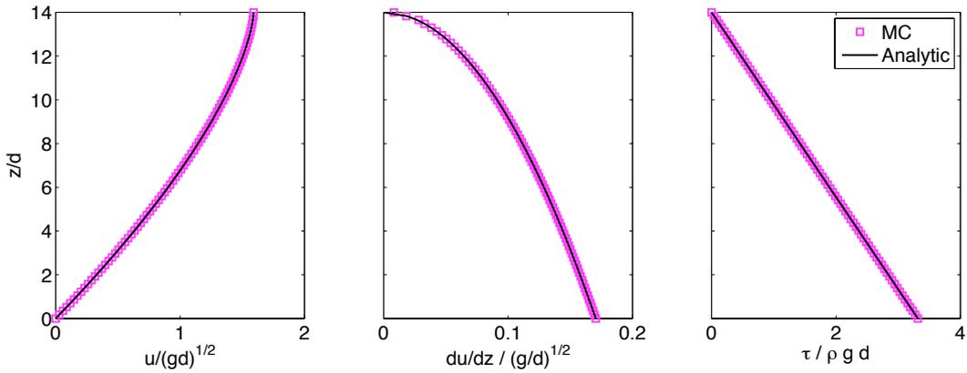
Figure 6: Granular flow over an inclined rough plane for  $\alpha = 0.406 \text{ rad}$  and  $H = 14$ . Comparison of computed ( $h = H/40$ ) and analytical solution profiles in the layer:  $u$ -velocity component (left), vertical velocity gradient  $du/dz$  (center) and shear stress  $\tau$  (right).
