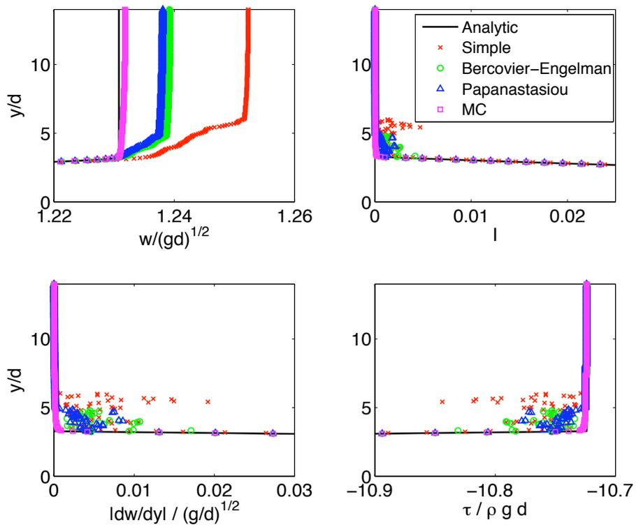
Figure 4: Vertical-chute flow test case with  $p = 28$  and  $b = 28$ . Comparison of computed ( $h = b/320$ ) and analytical solution profiles: vertical velocity component  $w$  (upper left), transverse velocity gradient  $dw/dy$  (lower left), inertial parameter  $I$  (upper right) and shear stress  $\tau$  (lower right).
