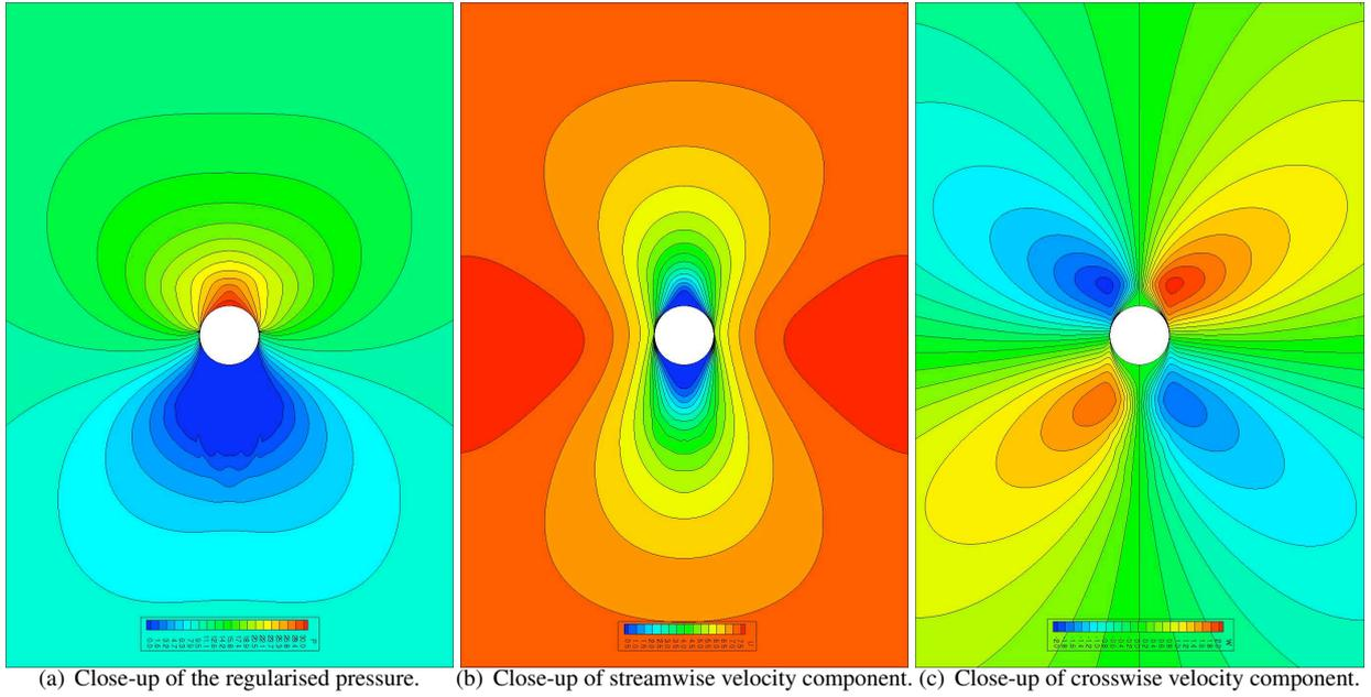
Figure 14: Granular chute flow around a cylinder, close-up in the vicinity of the cylinder of the iso-values of the primary variables for a dimensionless external loading of  $F_{adim}^v = 0.054$ .
