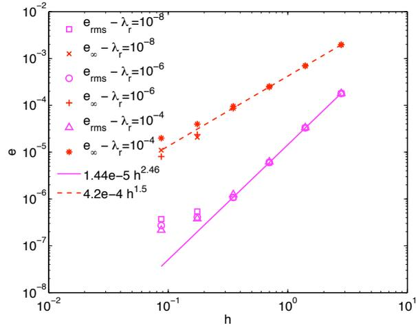
Figure 7: Granular flow over an inclined rough plane for  $\alpha = 0.406$  rad and  $H = 14$ . Spatial convergence analysis of the numerical solution in terms of RMS error and infinity norm. The RMS error is defined as  $e_{rms} = 1/N \sqrt{\sum_N (u_i - u_i^{ex})^2}$  and the infinity norm is defined as  $e_{\infty} = \max_N |u_i - u_i^{ex}|$ .
