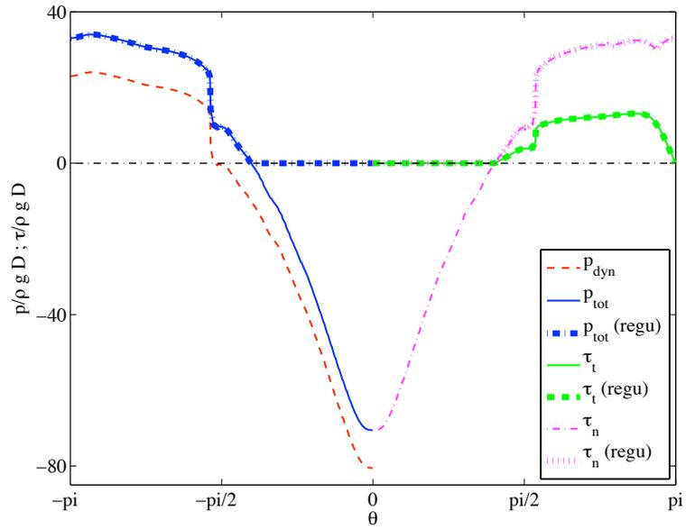
Figure 15: Granular chute flow around a cylinder for  $F_{adim}^v = 0.054$ . Plots along the cylinder perimeter versus the azimuthal angle of the dynamical pressure, total pressure, regularized one (plotted for  $-\pi \leq \theta \leq 0$ ), normal and tangential stresses and their regularised counterparts (plotted for  $0 \leq \theta \leq \pi$ ).
