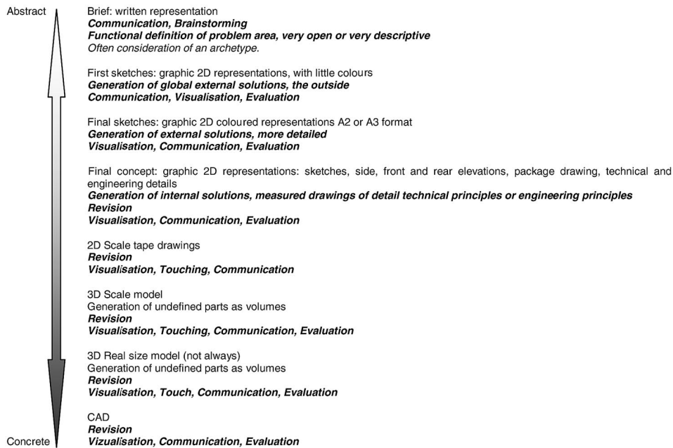
Figure 6 Transformation of the representation levels and their function in the traditional process
