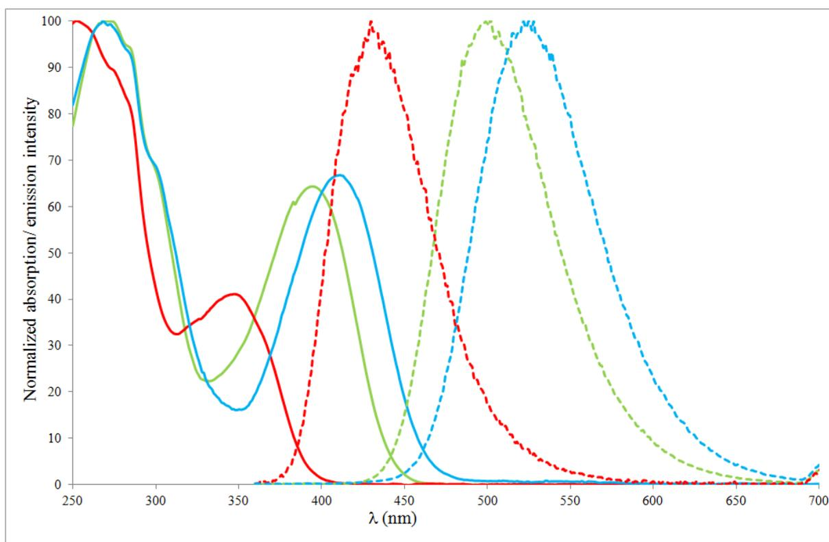
**Figure 1: Normalized UV/vis (solid line) and emission spectra (brocken line) of compounds 5d (green), 6a (red) and 6d (blue).**
