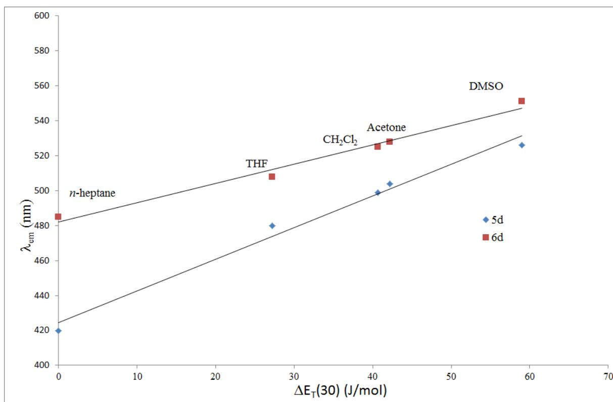
**Figure 7:** Emission wavelength ( $\lambda_{max}$ ) as a function of Dimroth-Reichart polarity parameter for compounds 5d and 6d.
