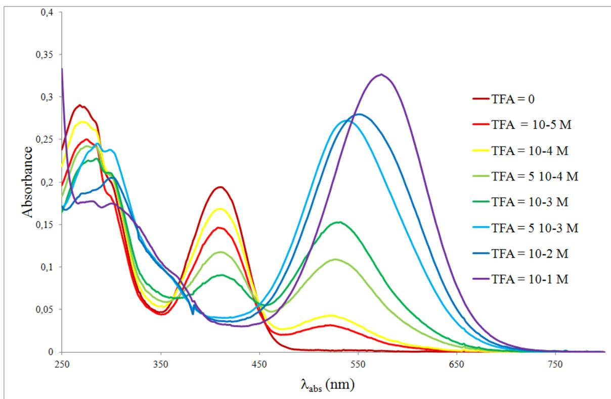
**Figure 4. Change in the absorption spectra of 6d ( $c = 1.2 \cdot 10^{-5}$  M) upon addition of TFA ( $10^{-5}$  M to  $10^{-1}$  M)**
