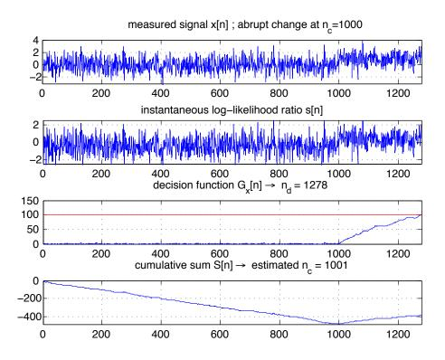
Figure 1.2: typical behaviour of the suboptimal CUSUM algorithm in the case of an iid Gaussian signal with a change in the mean at time  $n_c = 1000$ .
