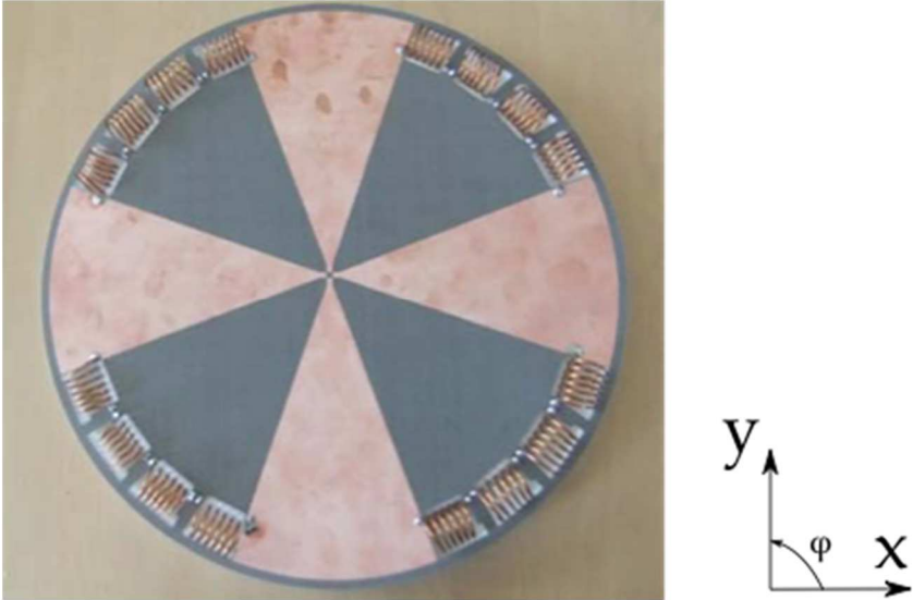
Fig. 4 - The proposed dual-linear polarized UWB antenna.
