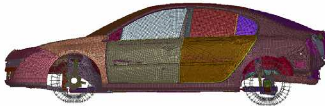
Figure 5 FE model of the vehicle before Craig and Bampton dynamic condensation
