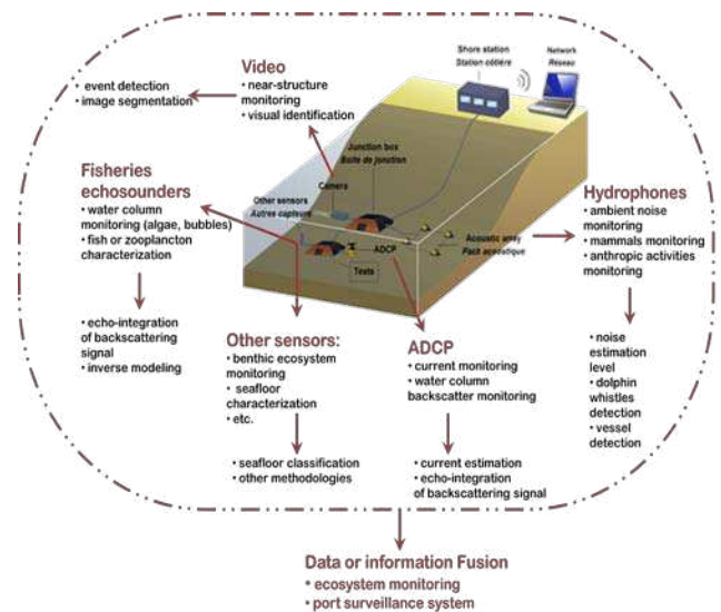
FIG. 1 SCHEMATIC OF OUR SURVEILLANCE SYSTEM
