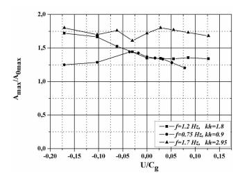
**Fig. 6.** Dependence of the amplitude in the focusing point on velocity of hydrodynamic flow for frequency modulated wave train:  $f_{\text{max}} = 0.75 \,\text{Hz}$ ,  $f_{\text{max}} = 1.2 \,\text{Hz}$  and  $f_{\text{max}} = 1.7 \,\text{Hz}$ .
