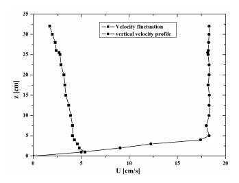
**Fig. 3.** Profiles of current velocity: mean profile and mean root velocity fluctuations at 3 m from the wave maker.
