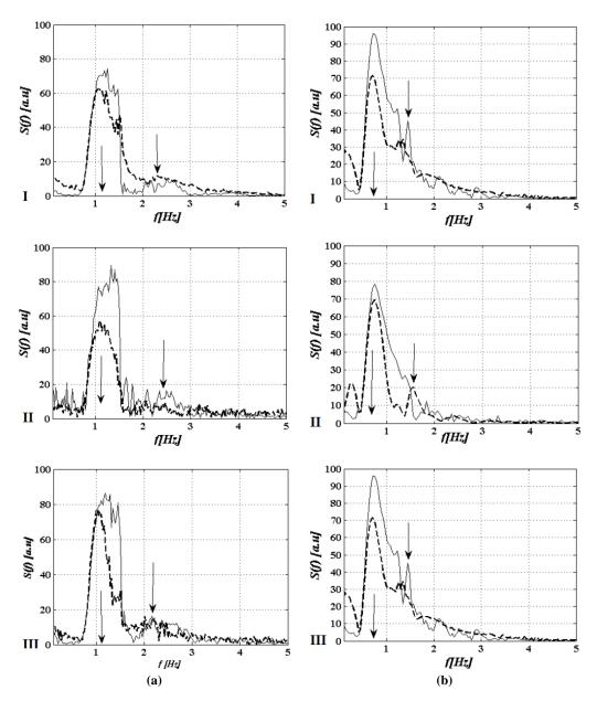
**Fig. 8.** (a) Comparison of spectra S(f) (arbitrary units) at distance x=0 (solid curve) and x=6 cm (dotted curve for  $f_{\rm max}=1.2$  Hz: (I) U=0, (II) U=0.12 m s<sup>-1</sup>, (III) U=-0.12 m s<sup>-1</sup>). (b) Comparison of spectra S(f) (arbitrary units) at distance x=0 (solid curve) and x=6 cm (dotted curve for  $f_{\rm max}=0.75$  Hz: (I) U=0, (II) U=0.12 m s<sup>-1</sup>, (III) U=-0.12 m s<sup>-1</sup>).
