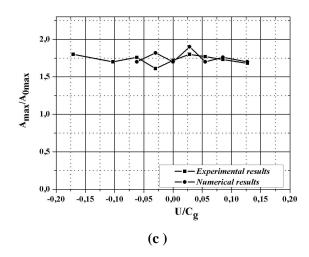
**Fig. 10.** Comparison of experimental and numerical results on amplitude in the focusing point for wave train (a)  $f_{\rm max}=0.75\,{\rm Hz}$ , (b)  $f_{\rm max}=1.2\,{\rm Hz}$  and (c)  $f_{\rm max}=1.7\,{\rm Hz}$ .
