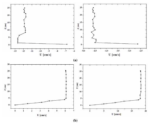
Fig. 4. (a) profiles of velocity for negative current in the vicinity of wave maker. (b) profiles of velocity for positive current in the vicinity of wave maker.
