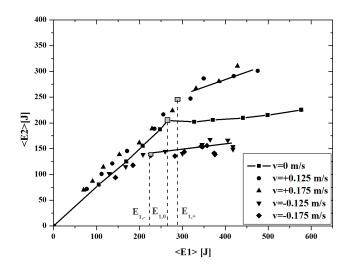
**Fig. 2.** Dependence of low frequency ( $f_{\text{max}} = 0.75$ ) wave packet energy  $E_2$  (energy measured at x = 15 m) on  $E_1$  (energy measured at x = 1 m).
