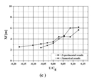
**Fig. 9.** Comparison of experimental and theoretical results on focusing point for wave train with (a)  $f_{\rm max}=0.75\,{\rm Hz}$ , (b)  $f_{\rm max}=1.2\,{\rm Hz}$  and (c)  $f_{\rm max}=1.7\,{\rm Hz}$ .
