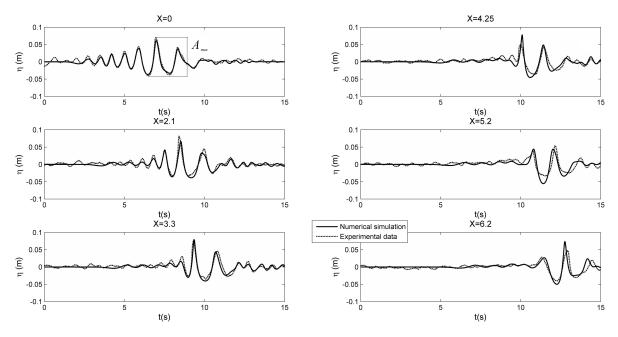
Fig. 5. Space—time evolution of impulse generated by wave maker. Dotted curves correspond to experimental data, solid curves are results of numerical simulations.
