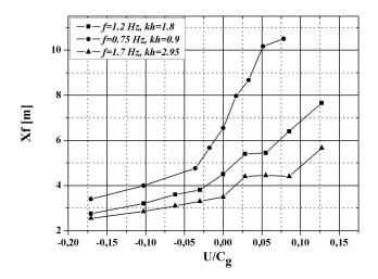
**Fig. 7.** Dependence of focusing point position on velocity of hydrodynamic flow for frequency modulated wave train:  $f_{\text{max}} = 0.75 \,\text{Hz}$ ,  $f_{\text{max}} = 1.2 \,\text{Hz}$  and  $f_{\text{max}} = 1.7 \,\text{Hz}$ .
