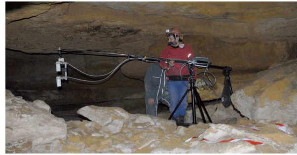
Figure 4. Measurements of magnetic field in the cave Les Fraux, using a dual sensor magnetometer fixed on a tripod (non invasive equipment).
