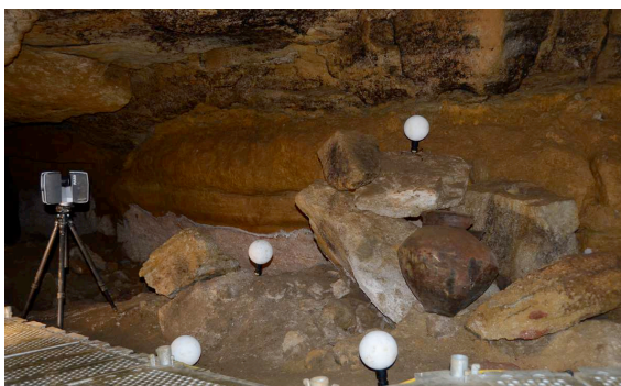
Figure 3. 3D-recording of a Bronze age ceramic deposit (using the Faro Focus 3D).
