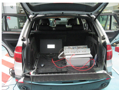
(a) Integration of the SDR platform on a BMW X5 test vehicle
