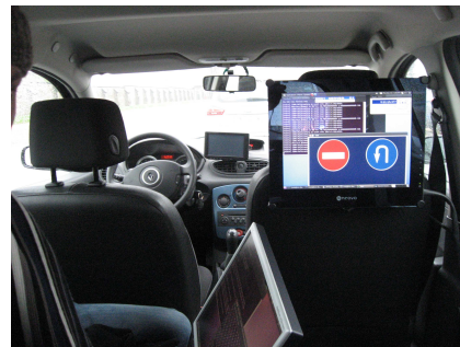
(b) Warning displayed on the vehicle driving on a wrong direction
