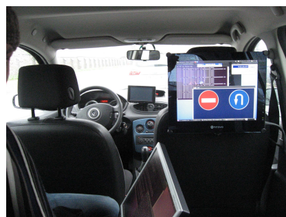
(b) Warning displayed on the vehicle driving on a wrong direction
