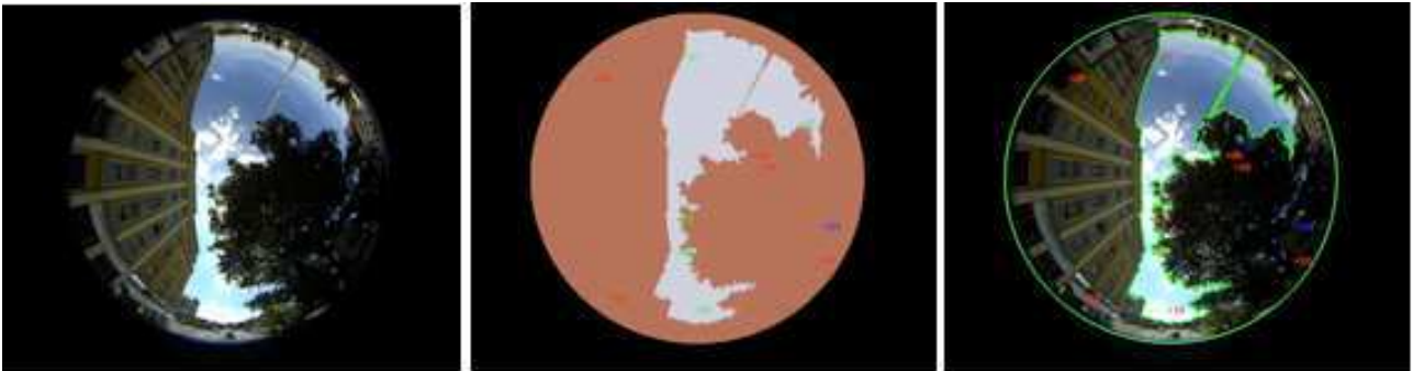
Figure 5: Example of image, its classification and satellite states of reception (source: [CAPLOC project])
