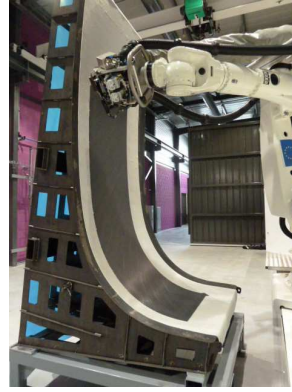
Fig. 18: Robot and landing gear door mold.
