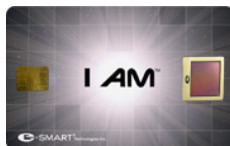
Figure 4: An example of a contactless smartcard for logical access control with an embedded fingerprint sensor for match on card (E-smart Technologies).
