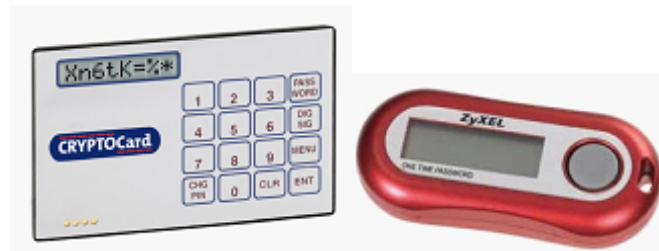
Figure 3: Left token is a challenge type OTP card with a PIN code (CRYPTOCARD © ). The one on the right is a counter synchronised OTP token (ZyXEL).
