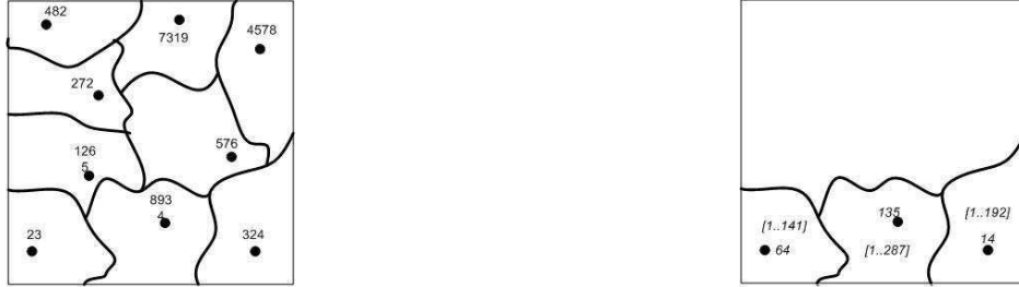
Figure 7. Division of the graph into disjoint clusters and local initialization of each cluster. In the figure on the right above, 3 clusters are initialized with integers ranging from 1 to 141, from 1 to 287, and from 1 to 192, respectively.
