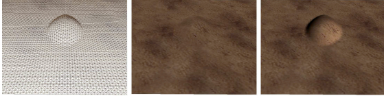
Figure 7: Left: displaced wireframe mesh; center: same mesh with texture applied but no normal correction; right: same mesh with texture and normal correction.
